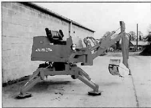
Upper structure offset for close wall digging or sideways digging
