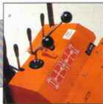
TWO LEVERS CONTROL ALL DIGGING FUNCTIONS
